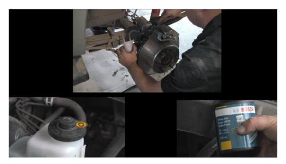
Adjust the handbrake shoes to the required tension via the access port in the backing plate. #20
