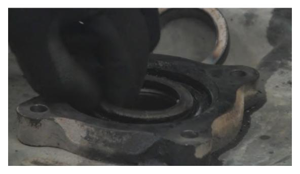
Remove the housing from the backing plate and using a press, remove the old wheel bearing.
