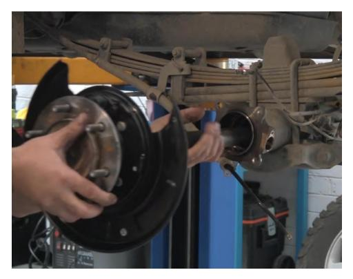
If any oil has leaked from the axle while disassembled, top up the diff oil now.
