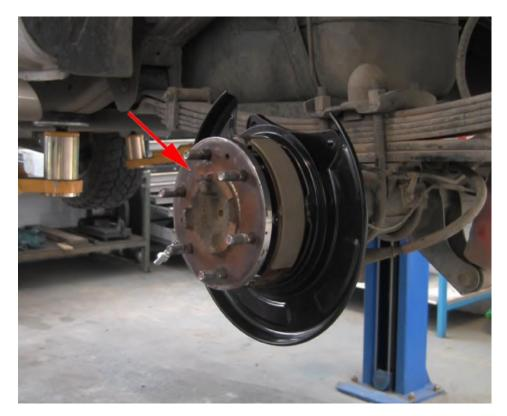
Fit the new brake rotor.
