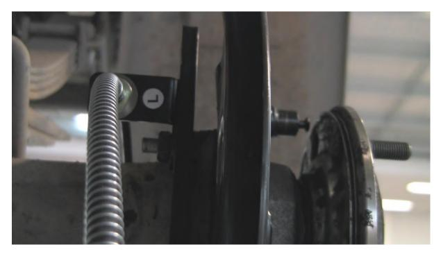
Fit the brake hose kit #4 to the caliper bracket #7.
