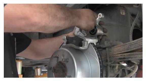
Remove clamps from flexible brake hose.
