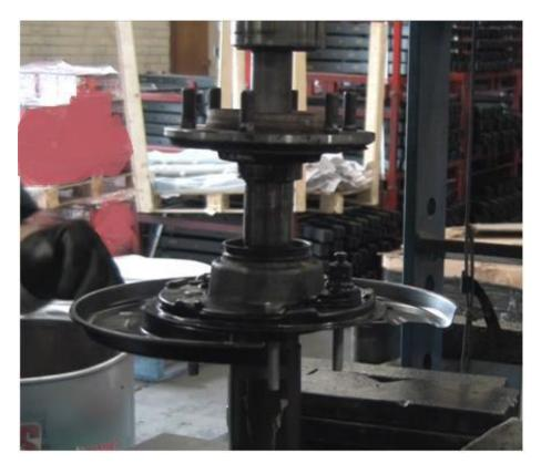
Replace the circlip.
