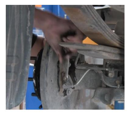
Remove the handbrake retaining clip and cable.
