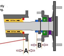
Remove the O ring seal from the axle.
