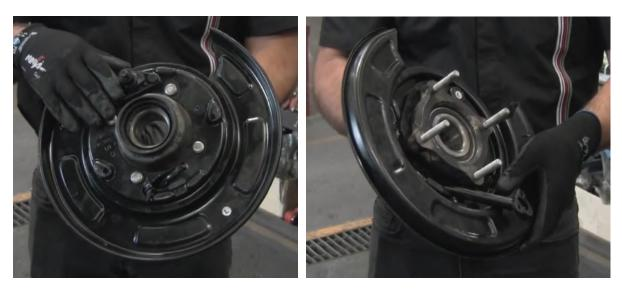
Take the assembly back to the press and press the axle into the hub.
