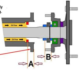
Replace the axle assembly back into the housing, taking care not to damage the inner seal.
