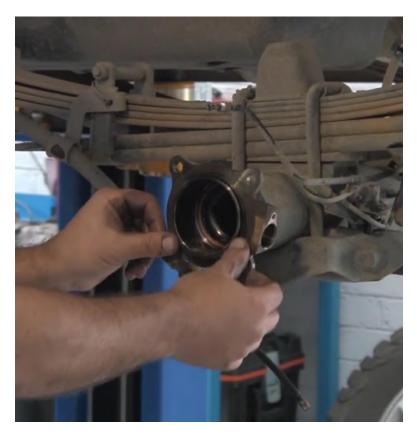
It is critical to ensure that the inner axle seal contacts the centre of the axle collar. This may mean that the collar is not pressed hard against the ABS ring during assembly.
