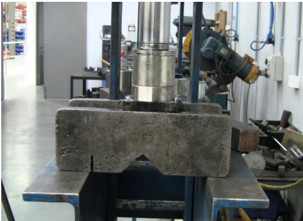
Place the new backing plate onto the housing and then press the new studs into the bearing housing.
