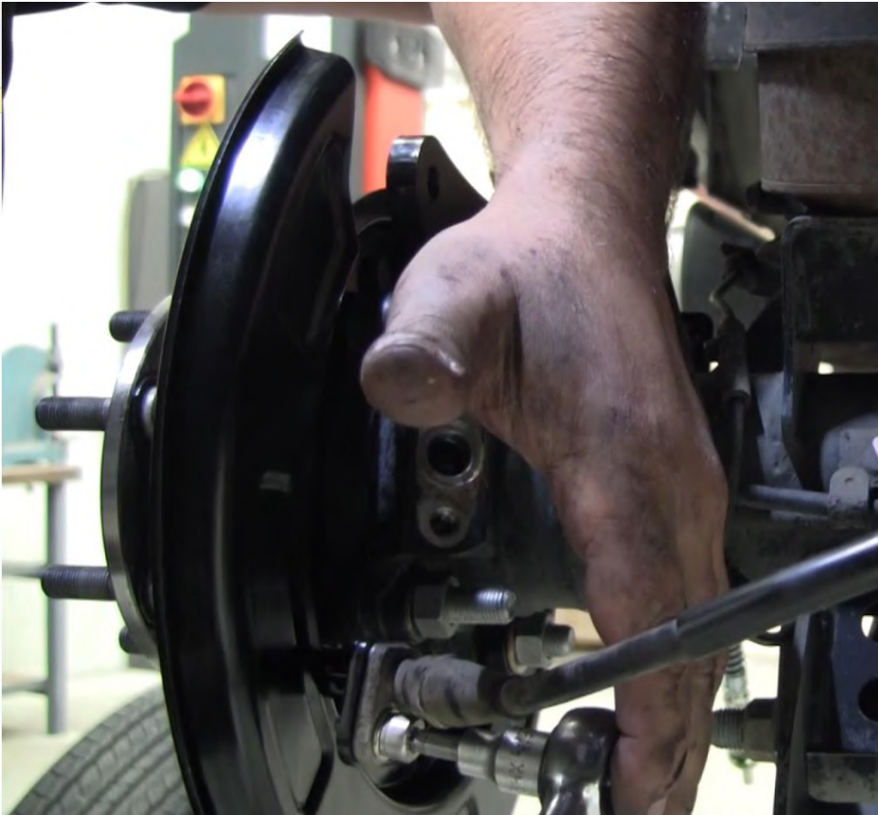
Fit the new handbrake assembly and refit the cable. #9 & #22
