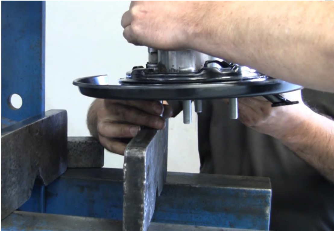
Press the backing plate and bearing housing onto the axle. #24
