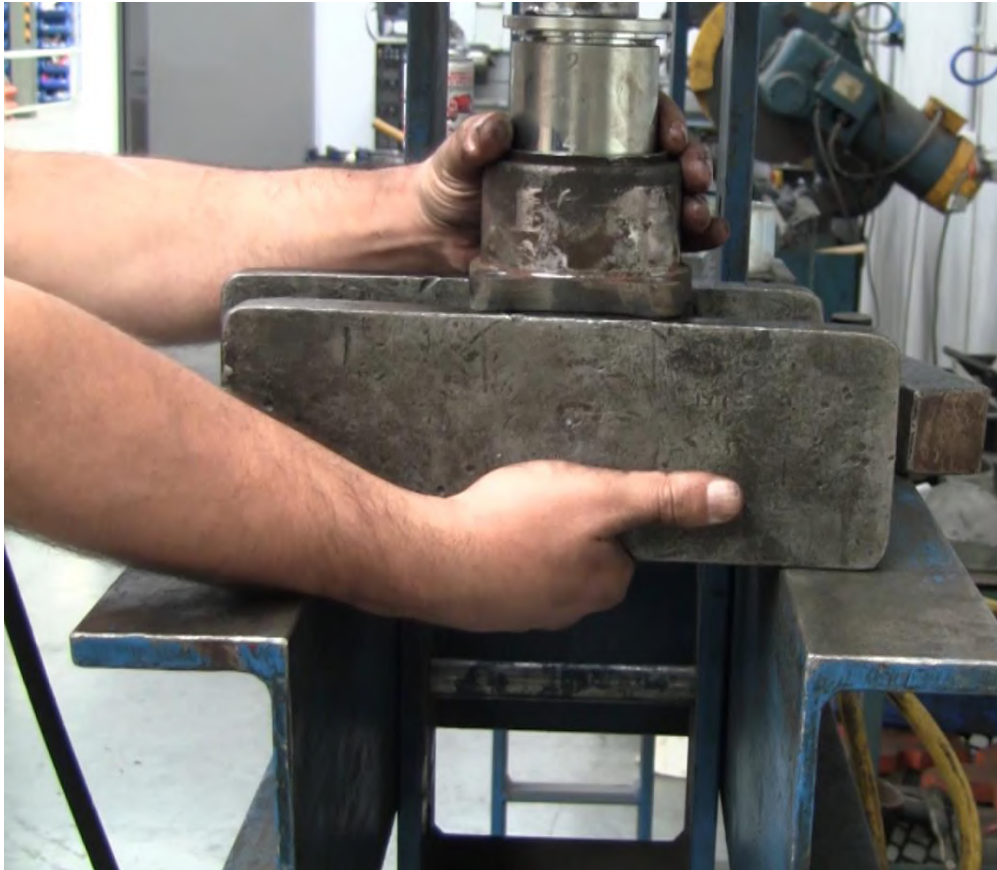
Press the supplied new bearing into the housing. #16
