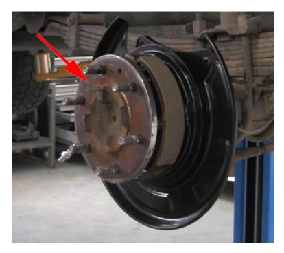
Fit the new brake rotor
