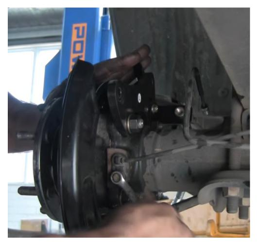
Refit handbrake assembly and handbrake cable onto the backing plate. #9 & #22  $\,$
