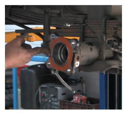
If any oil has leaked from the axle while disassembled, top up the diff oil now.
