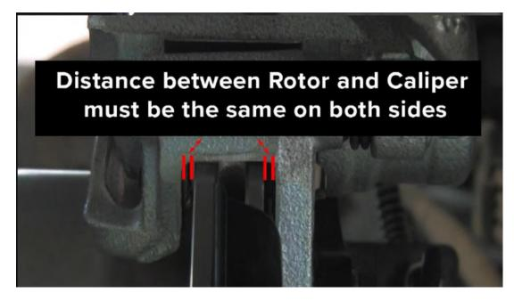
Apply LOCTITE and tighten cradle mounting bolts and recheck alignment.
