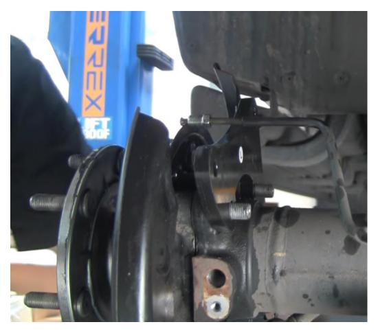
Place the brake hose bracket #4 onto the stud ensuring they are on the correct side of the vehicle.
