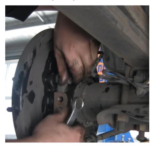
Remove the four axle flange mounting nuts.
