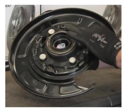
Place the inner bearing race onto the bearing housing and then the completed assembly onto the axle. Use the press to complete the operations.
