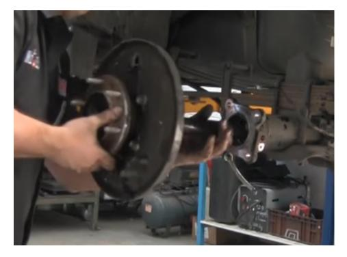
Remove the circlip, holding the tone wheel.
