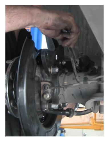
Before fitting the new brake rotor, make sure the axle face is clean.
