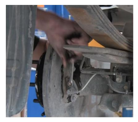
Remove the handbrake retaining clip and cable.
