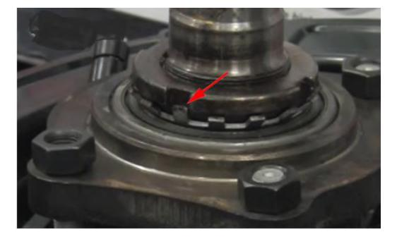
When the locking nut is in place, bend the tab to lock it in place.
