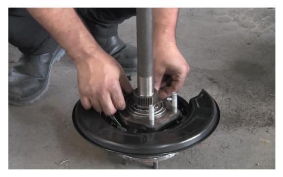
Replace the axle assembly back into the housing, taking care not to damage the O ring seal.
