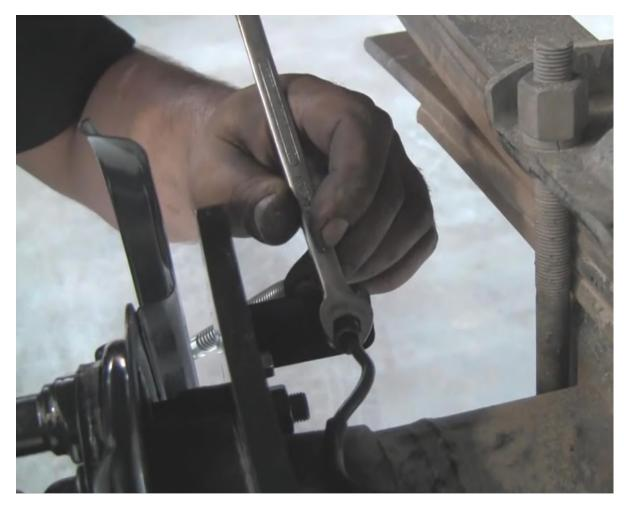
Fit the new handbrake assembly and refit the cable. #9 & #22
