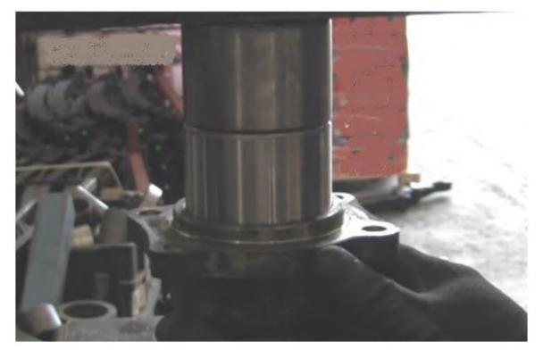
Press the new studs into just the bearing housing for the splines to create new grooves.
