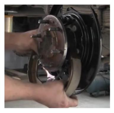
Before fitting the new brake rotor, make sure the axle face is clean.
