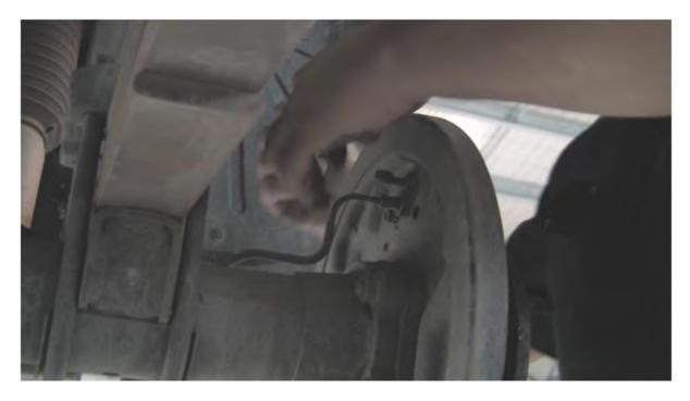
Carefully remove the ABS sensor and place it out of way.
