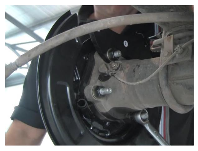
Refit the handbrake cable to the backing plate. #26
