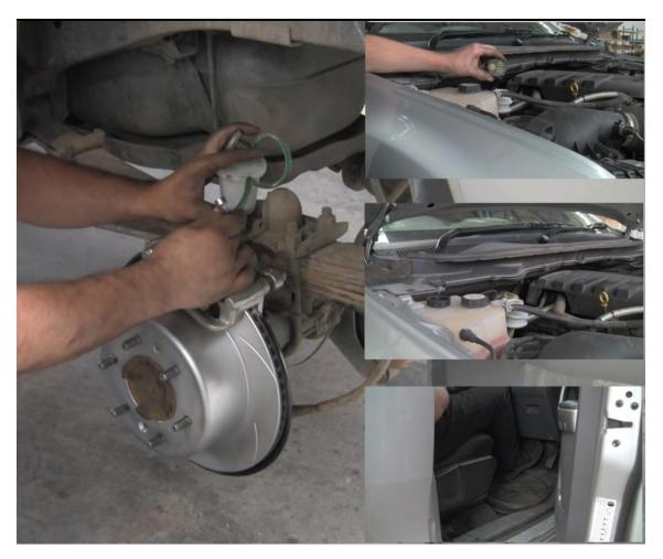
Adjust the handbrake shoes to the required tension via the access port in the backing plate. #20
