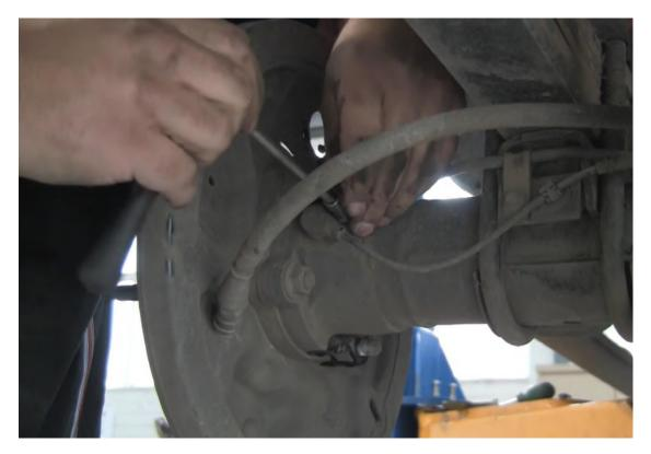
Remove the handbrake retaining clip and cable.
