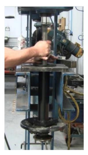
Then remove the bearing from the housing.
