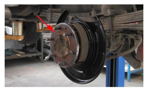
Fit the new brake rotor and secure with the supplied screws. #25
