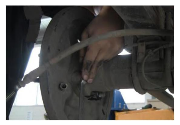
Remove the axle from the vehicle.
