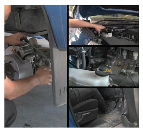
Adjust the handbrake shoes to the required tension via the access port in the backing plate. #20
