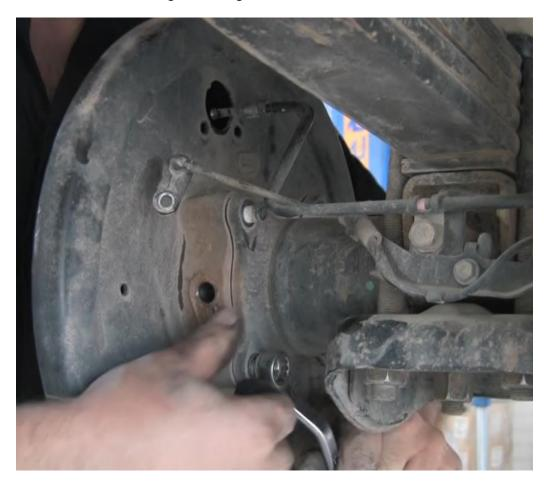
Remove the axle from the vehicle.
