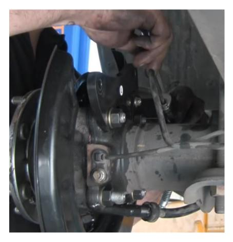
Before fitting the new brake rotor, make sure the axle face is clean.
