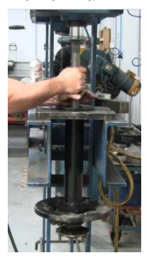
Remove the collar and spacer noting the orientation.
