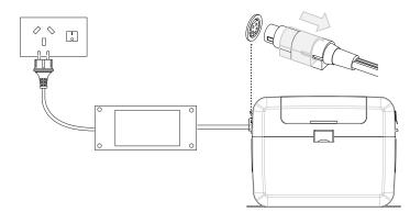
240V AC or 12V DC Secure Connection - Simply pull back the plug sleeve, insert, then release. This locks the lead into the Hulk Powerpack for a secure fit in all situations - especially on the move
